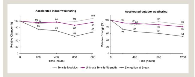
Note: For the indoor method, it is possible to infer that accelerated weathering times of 400 and 800 hours correspond to ca. 5 and 10 years of ageing in normal conditions, respectively. For the outdoor method, it is possible to infer that accelerated weathering times of 600 and 1200 hours correspond to ca. 12 and 24 months of ageing in normal conditions, respectively.
